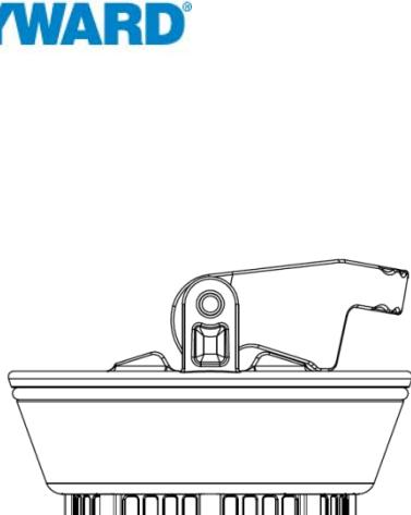
Fig. 5: Handle in "locked" position
