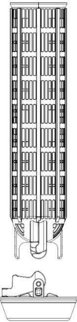
Fig. 11C: Basket ring removed from basket (side view)
