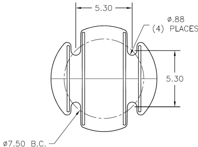
Fig. 1: FLV-Series base mounting pad
