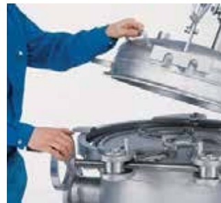
3. Open the cover aided by spring-assisted mechanism.
