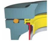
SENTINEL filter bags utilize a pressure activated sealing lip, which responds to increases in differential pressure
