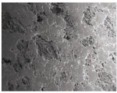
Surface of a MAX-LOAD pleated filter bag
