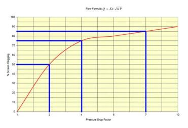
In practice this means that, assuming a consistent particle size and volume, the amount of time required to become 75% clogged is only ½ the time required for the initial 50% clogging. Stated another way, once you reach 50% clogged, the clogging rate doubles.
