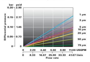
High differential pressure can result in a reduction in flow rate or result in an increase of the energy required to maintain a steady flow rate.
