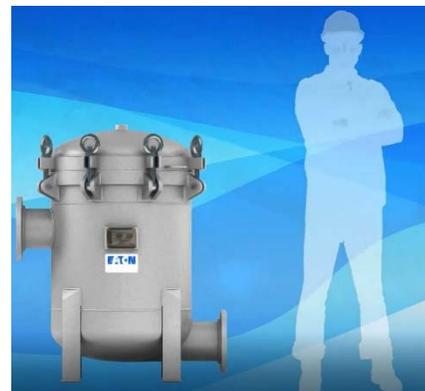
They also both have a swing eyebolt closure (rated for pressures up to 150 PSIG at 200°F.), enabling quick access to the filter bags, generally within 1-2 minutes, and provides a firm seal with minimal effort. The spring assisted counter weight closure of both MAXILINE and PROLINE enable one handed opening and it remains at any position for safer access to the filter bag chamber.
