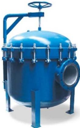
The MAXILINE HD has a swing bolt closure lifted by a handwheel driven lifting davit, a requirement for filter housings having 14+ filter bag chambers because the closure for housings that large is too heavy for spring assisted hinged closures used by the other vessels. Available in both 304 SS and carbon steel materials, its custom fabricated design enables customizations such as oversized inlet/outlet nozzles.
