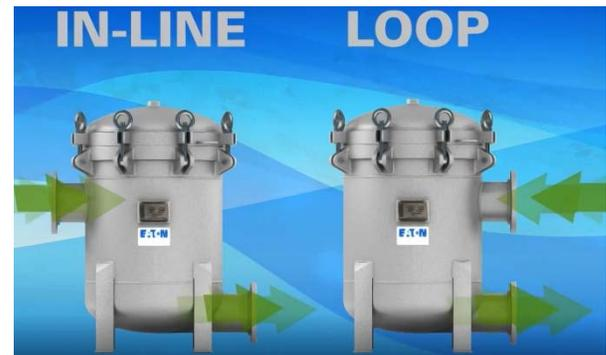
PROLINE bag filter housings are made of 304 stainless steel in both in-line and loop flow path configurations. Both MAXILINE and PROLINE bag filters have their outlet nozzle mounted tangentially to the dish shaped bottom, minimizing the vessel height in support of comfortable ergonomics and reduced risk of injury when removing full filter bags because ladders and stools are not required.
